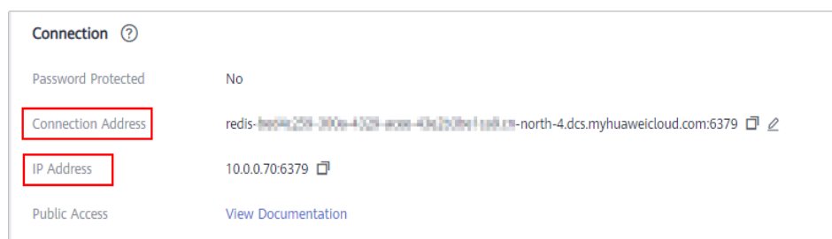
Figure 6-2 Obtaining the instance connection addresses
